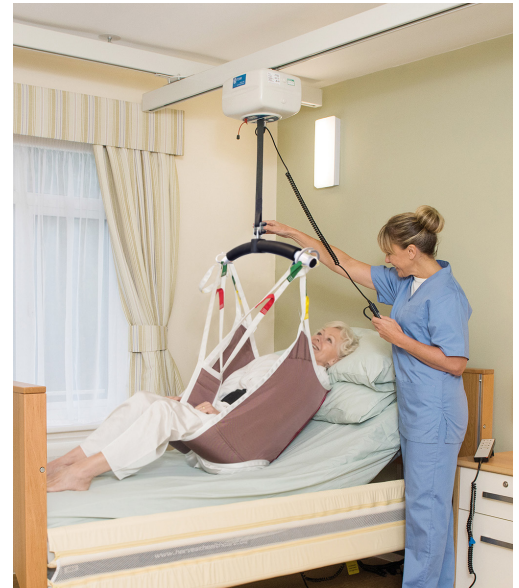
Person being assisted in using a ceiling hoist with sling and spreader bar.
